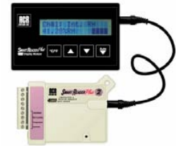
SRP Display Module (black) shown with an SRP data logger
