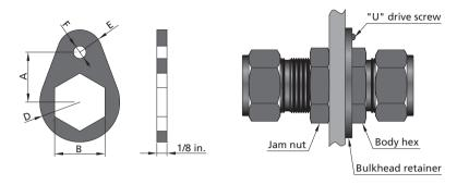
Bulkhead fitting installation utilizing bulkhead retainer
