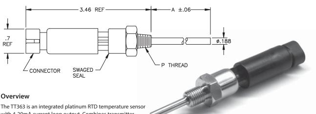
The TT363 is an integrated platinum RTD temperature sensor with 4-20mA current loop output. Combines transmitter capability with a platinum sensing element in a single package for an easier-to-install temperature sensing solution.
