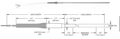
Probes can be bent around a mandrel diameter at least 3 times the probe diameter without kinking.
