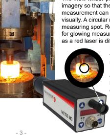
The **view finder** provides upright imagery so that the target under measurement can be viewed visually. A circular reticle shows the measuring spot. Recommended for glowing measurement objects, as a red laser is difficult to detect.
