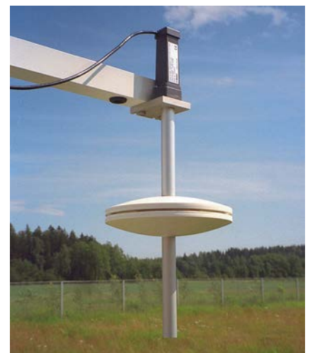
PTB210 paired with SPH10 static pressure head
