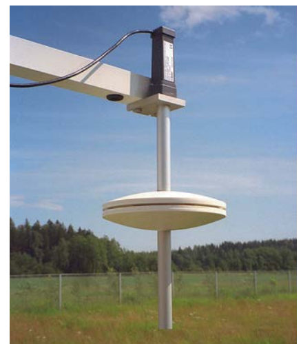
PTB210 paired with SPH10 static pressure head
