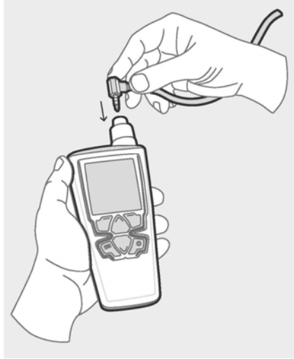
Snapping a connector to the indicator HM40 to read the measurement results.
