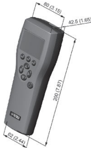
MI70 dimensions in millimeters (inches)
