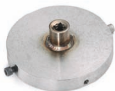
3½" Ring removal current design PN 101B221-01
