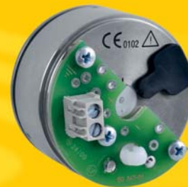
Wiring print with screw terminals
