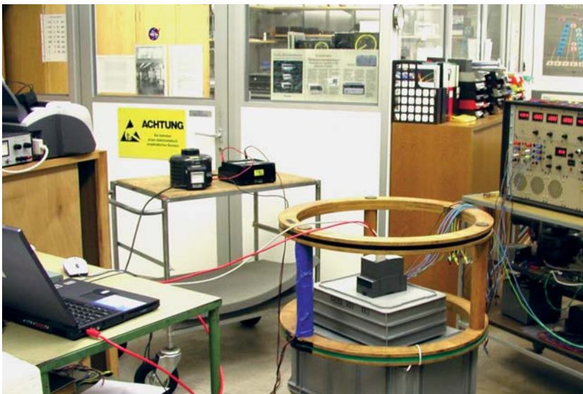
Determination of device behaviour under the influence of a magnetic external field generated by a Helmholtz coil
