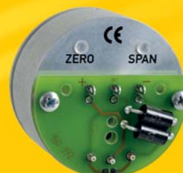
Wiring print with trans-zorb-diode
