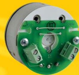
Wiring print with screw terminals
