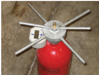
Fire Extinguisher Pressure Testing
