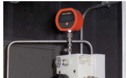
Industrial Gauge Manifold
