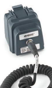
The Heise PTE-2 provides accurate temperature measurement when using the HM2-RT module with an RTD probe. This system supports the most common RTD's without requiring operator input of probe characterization data; each module comes factory-programmed with standard curves for Pt100 (385 & 392), Ni 120, Cu 10 and temperature probes.
