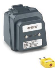
With the HM2-TC1 interface module installed, the PTE-2 contains programming to read types J, K, T, E, R, S, B and N thermocouples and display the measurement in units of temperature measure or millivolts. Other types of thermocouples may also be read by using the direct millivolt readout.
